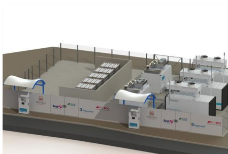
This graphic shows what the refuelling station at Kittybrewster depot in Aberdeen will look like, which also includes electrolyzers for producing the hydrogen.
